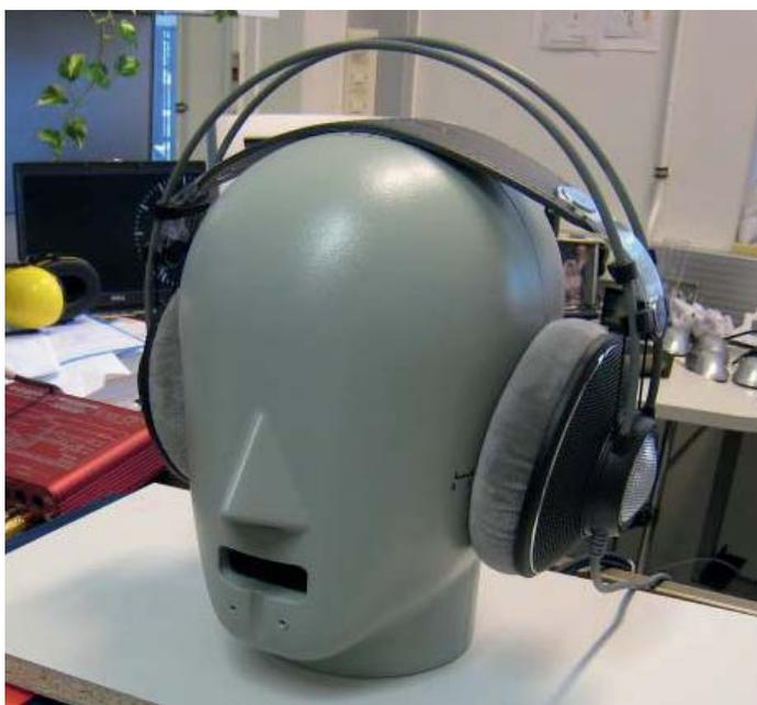
Fig. 4: Headphone calibration for listening tests by head simulator
