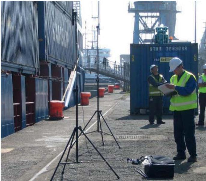
Fig. 1: Sound power measurements and recordings in the Port of Dublin
