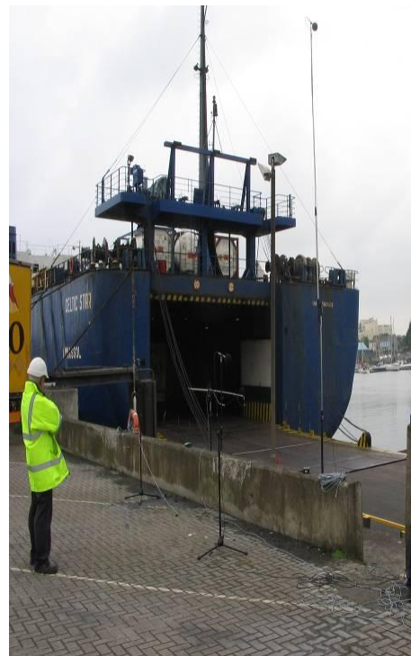
Figure 3: Measurement set up of a RoRo ramp.
