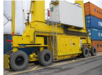
Figure 2: Measurement set up of an RTG power unit.
