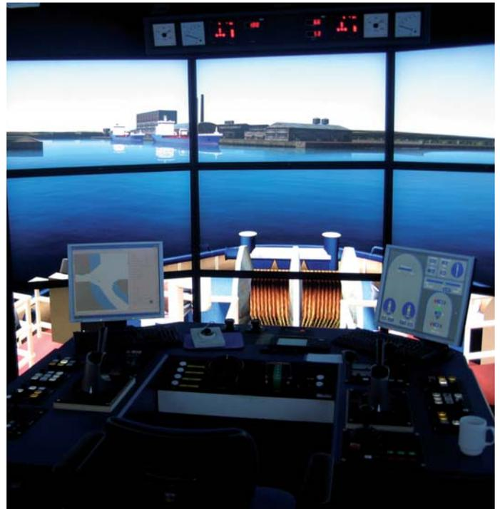
When tugs work in waves and push the side of a large assisted ship, large vertical friction forces may be generated, which may destroy the tug's fender. Such forces are not considered in present day's simulators. A fender simulation module was developed, which determines both the push force and the longitudinal and vertical friction forces. A side result of this module is that it may be used to simulate a grounding and a salvage operation.
