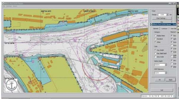
While the traditional ECDIS gives depths information only broadly between stepped depth contours lines, the PortECDIS displays very accurate depths contours and some single depths over the entire water area.
