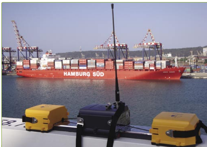
Figure 1. Prototype of portable pilot equipment (Sea Fix), providing the speed, positioning and heading information. Results are shown on a laptop display.
