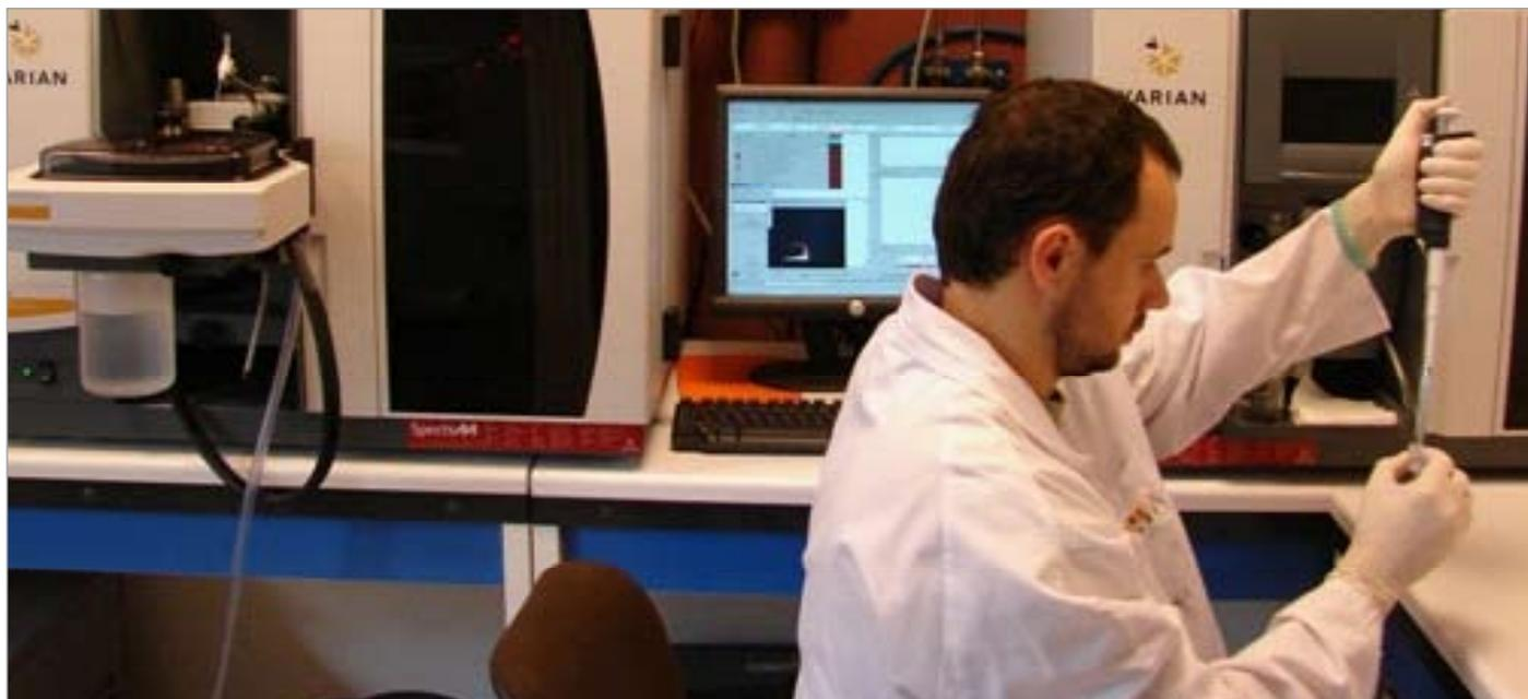
Flame Atomic Absorption Spectrometry for aluminium analysis from mussels
