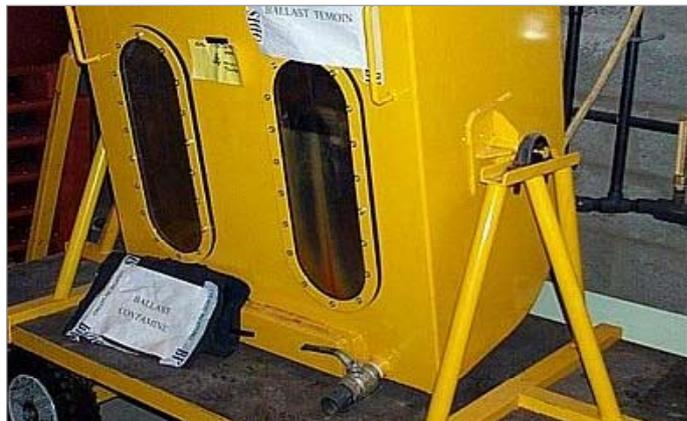
« Ballastodrome » developed by IFREMER for the test of biocide efficiency against organisms' mix
